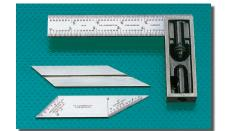
Double squares are popular with machinists, tool and pattern makers. Hardened, sliding blades are adjustable for a wide variety of uses. Faces of head are ground square. 6"/150mm size is equipped with a level, head is approximately 3-1/2" (90mm) long, and the faces approximately 9/16" (14mm) wide.
