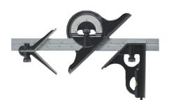
Hardened and Ground. Set includes 12" stainless steel chrome plated blade with 4R inch (8ths, 16ths, 32nds, 64ths) graduations, double indexed and reversible Protractor Head with full 180° graduation and spirit level, Square Head with level and scriber, and Center Head.
